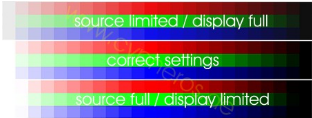
Illustration 17: Effect of a wrongly set “video_full_range_flag”
