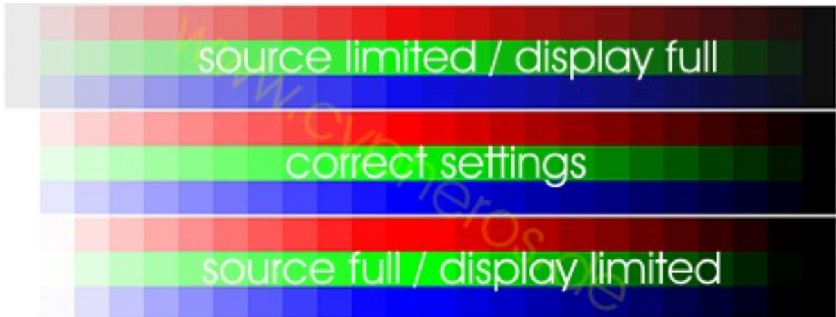
Illustration 17: Effect of a wrongly set “video_full_range_flag”
